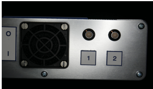
Blank LEDs during Initialisation
