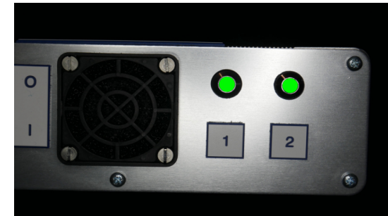
Two Green LEDs during Normal Operation
