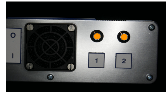
Two Green LEDs during Normal Operation
